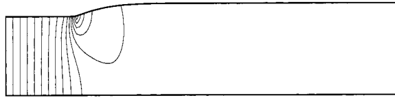
Figure 4. Pressure contours for the creeping Newtonian jet and Ca = 100 .
